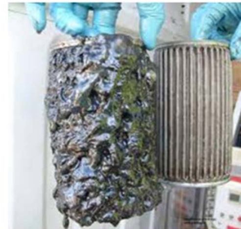
Clogged Station Dispenser Filter
