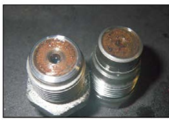
Water related corrosion
